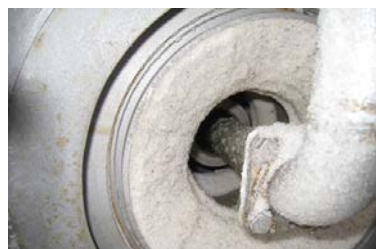
Figure 2.2 Pilot plant pusher centrifuge loaded with a cake from extraction
