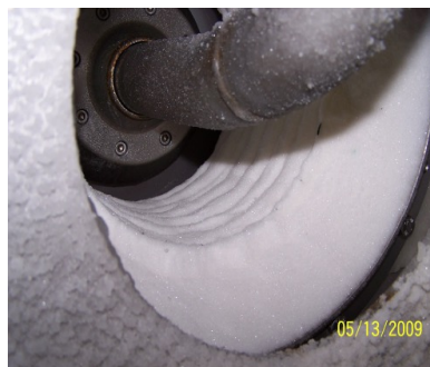
Figure 2.3 Pilot plant pusher centrifuge loaded with crude Epsom salt from crystallizer
